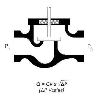
The  $\Delta P$  ( $P_1$ - $P_2$ ) across a conventional valve changes with system pressure fluctuations. Coil flow will vary regardless of changes in load.
