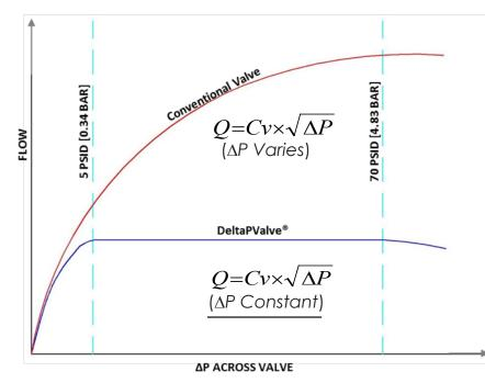
The  $\Delta P$  ( $P_1$ - $P_3$ ) across a conventional valve changes with system pressure fluctuations. Coil flow will vary regardless of changes in load.
