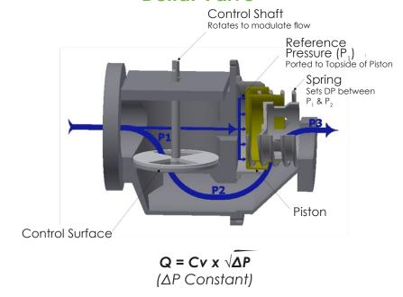
The  $\Delta P$  across the control surface  $(P_1-P_2)$  in a pressure independent DeltaPValve® remains constant despite system pressure fluctuations. Coil flow only varies when the actuator rotates the control shaft to accommodate changes in load.
