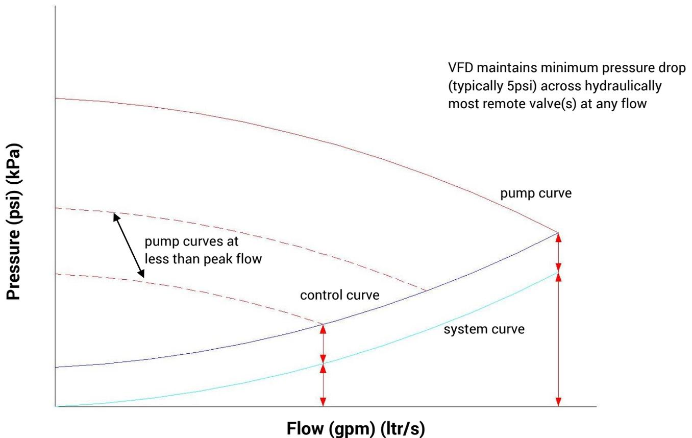
**Figure 5: Variable Speed Pumping**
