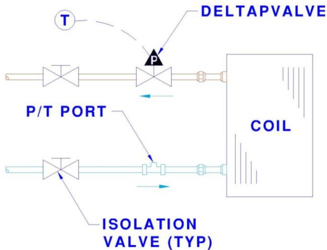
Return water temperature sensing to building management system (BMS) is recommended. Flow is directly related to actuator rotation position and is recorded on the valve tag.
