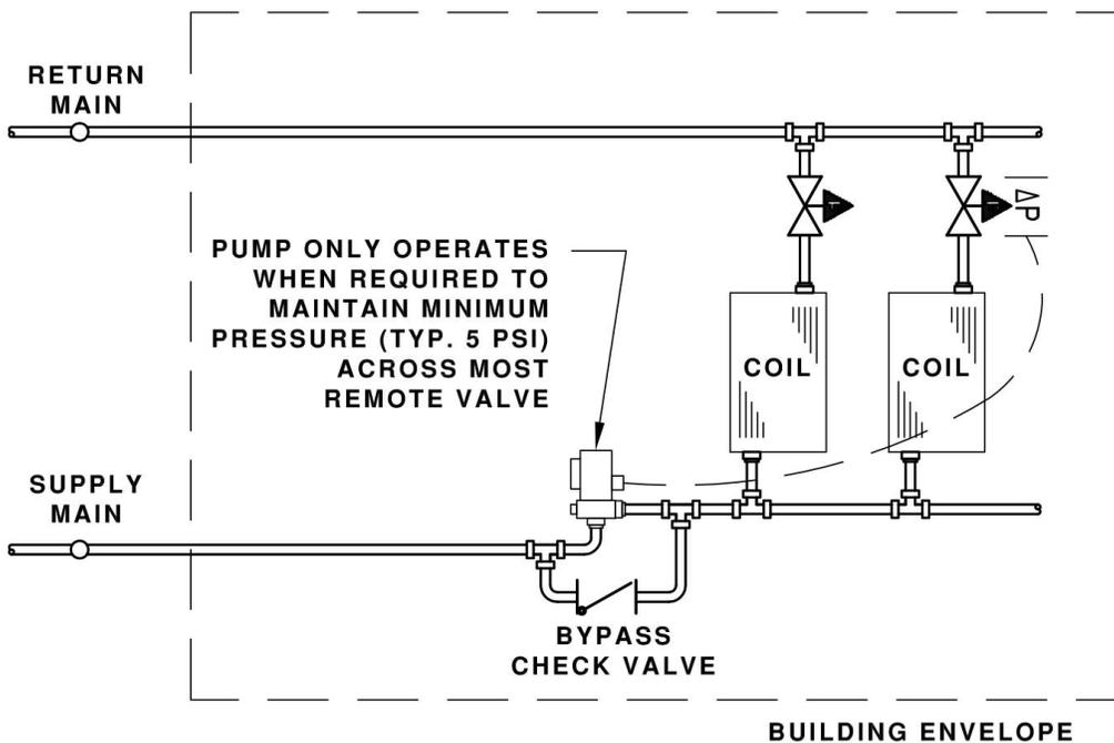
**NEW CONFIGURATION:** Minimum flow and design delta T are guaranteed higher at all load conditions (when chilled water is supplied at design or below and supply air temperature is set at design or above). Pump energy is dramatically reduced due to bypass and high delta T. DeltaPValve flow is controlled by thermostat. Humidity issues are solved.
