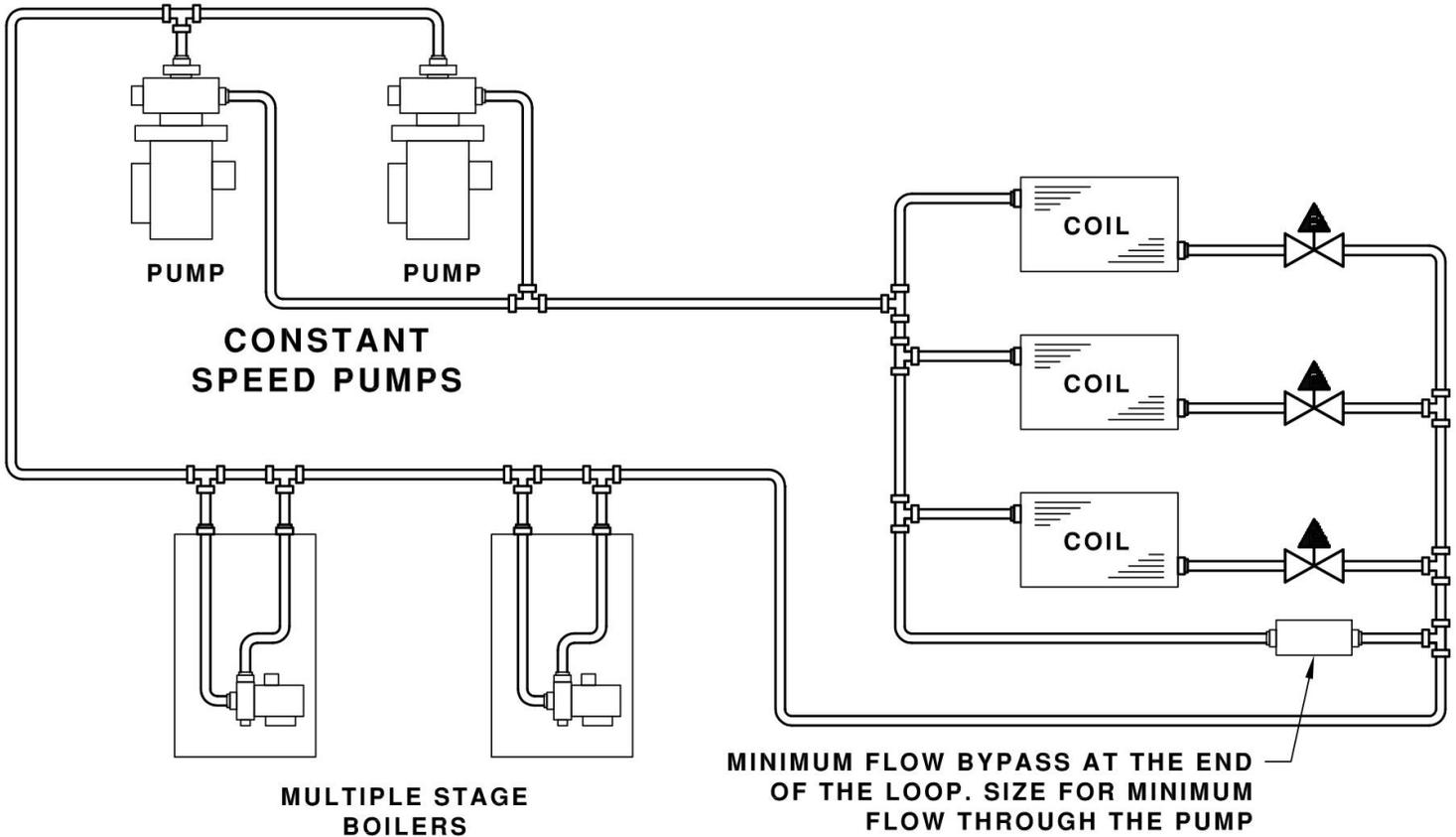
**Figure A1: Small Heating System - Constant Speed Pump**
