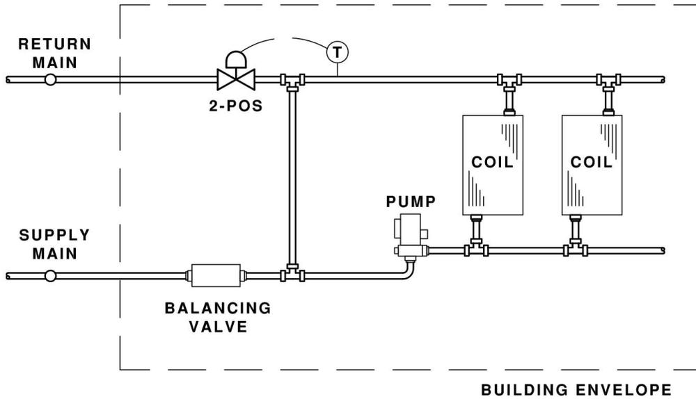
**EXISTING CONFIGURATION:** Excess flow and low delta T due to in-line pump and chilled water return blending with supply. This method wastes pump energy and creates humidity problems in the building.
