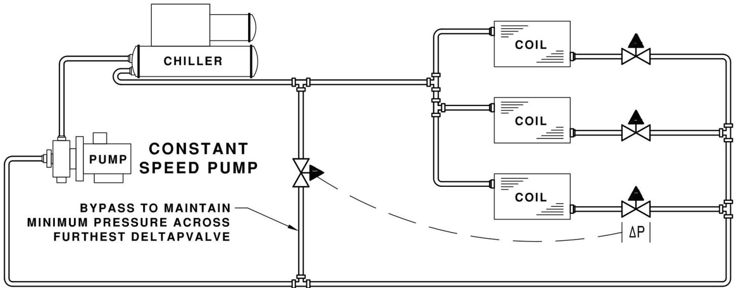
**Figure A4: Small Chiller System - Constant Speed Pump**
