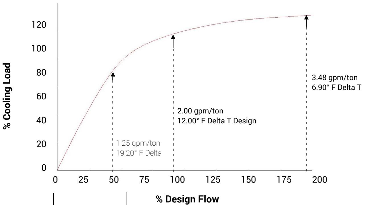
In HVAC hydronics systems, control valves must be able to operate properly at low flows and loads. They should operate in this % of design flow range the vast majority of the time.
