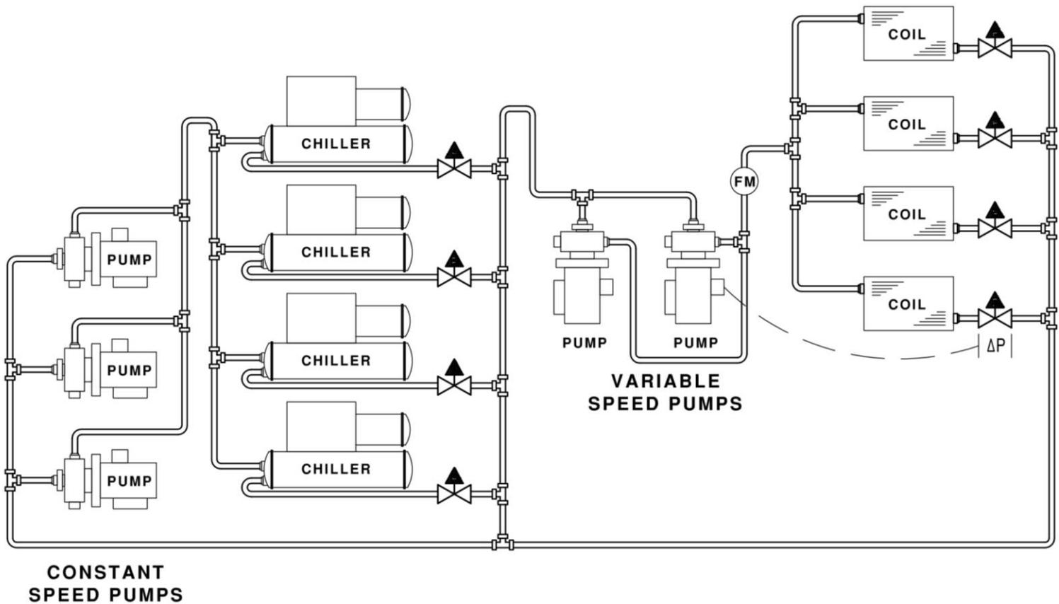
**Figure A6: Large Chiller Plant – Primary/Secondary Pumping**
