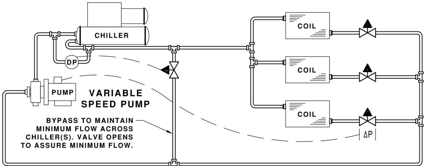
**Figure A5: Small Chiller System - Variable Speed Pump**
