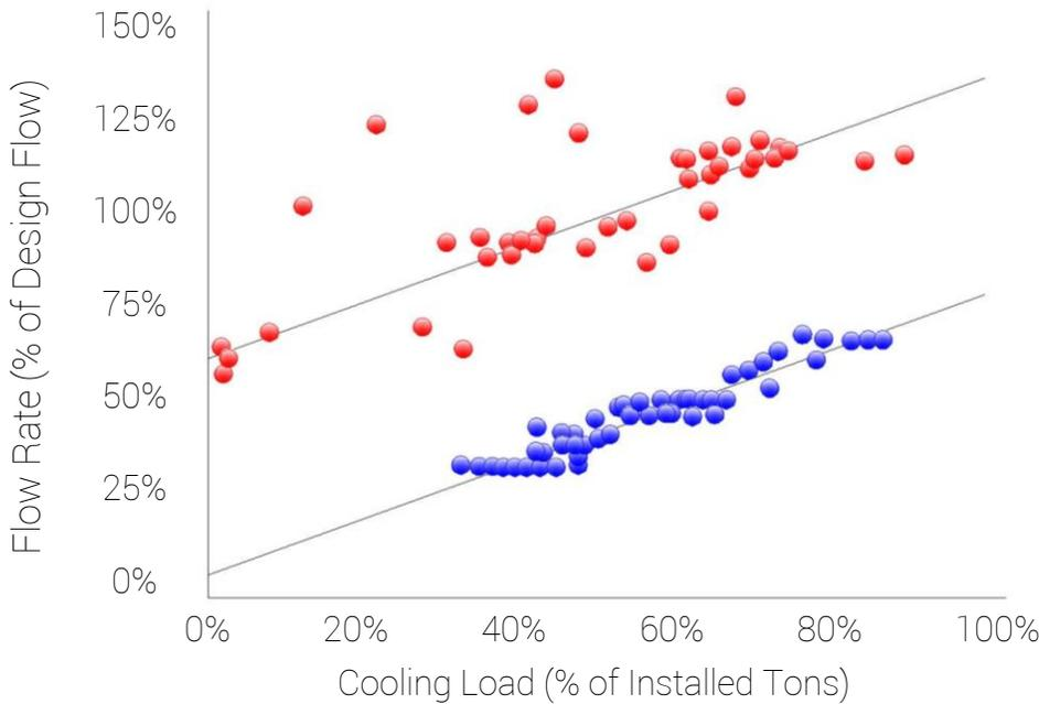
**Figure 1: % Cooling Load vs. % Flow Rate**
