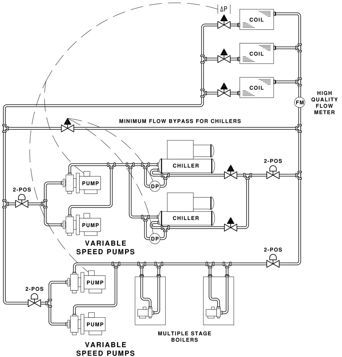
**Figure A9: Two-Pipe Changeover System – Excellent System for Schools**
