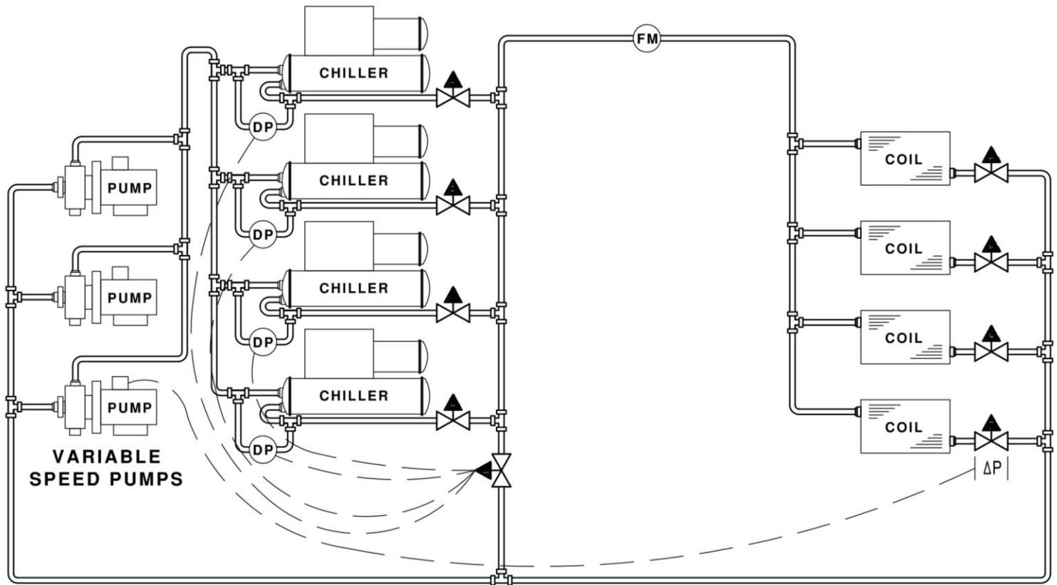
**Figure A7: Large Chiller Plant – Primary Variable Flow**
