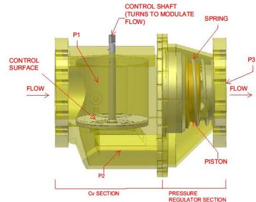
**Figure 6: DeltaPValve® Schematic**
