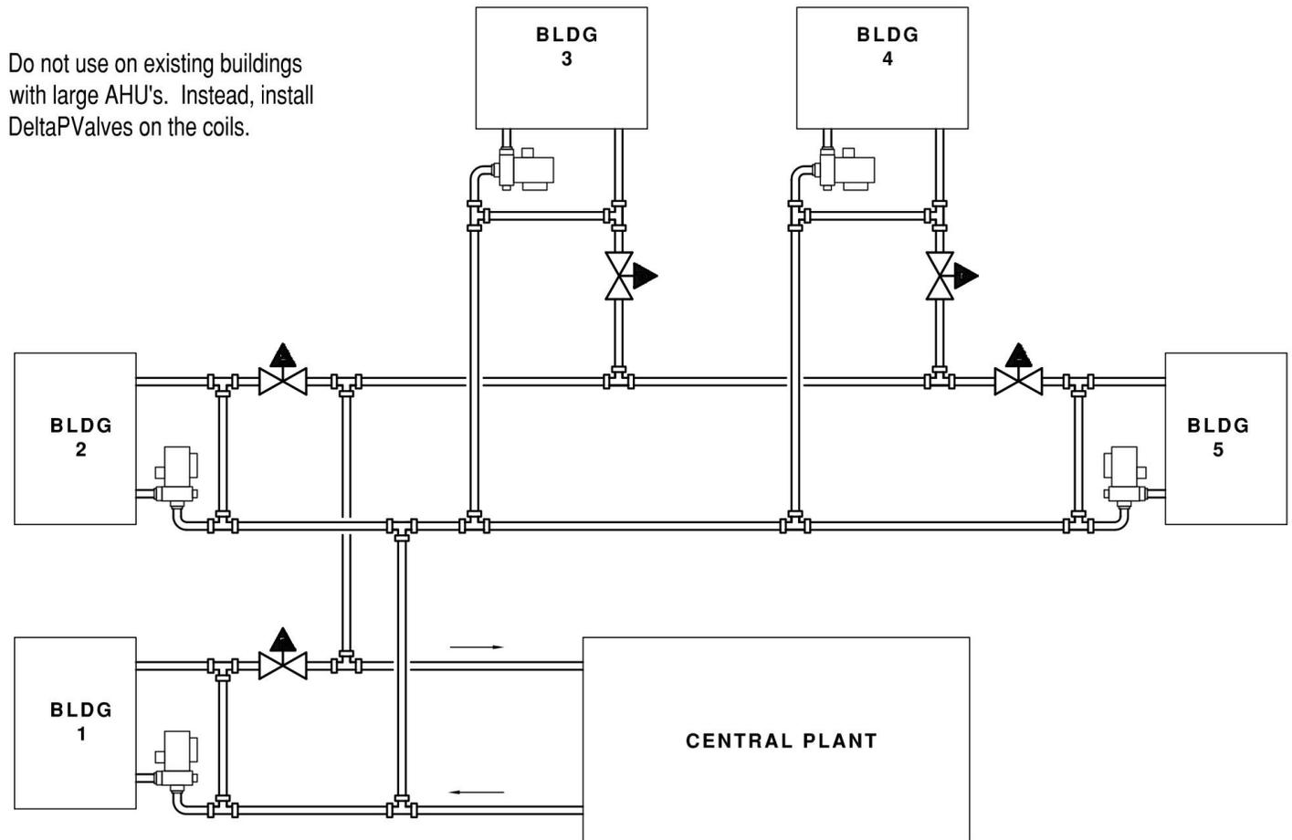
**Figure A8: Typical Campus Piping Schematic – Decoupled Buildings – With Many Small FCUs**
