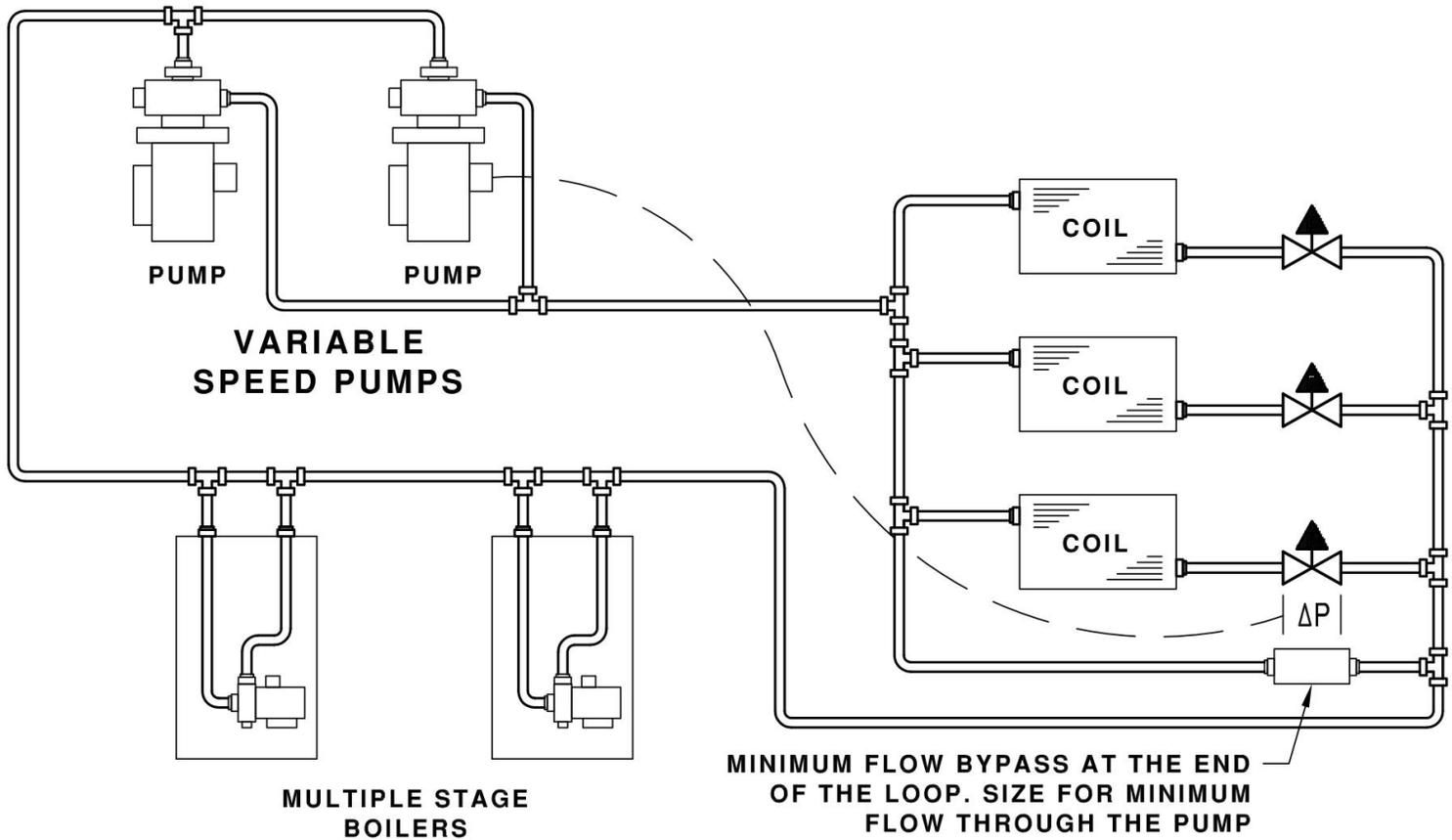
**Figure A2: Heating System – Variable Speed Pump**
